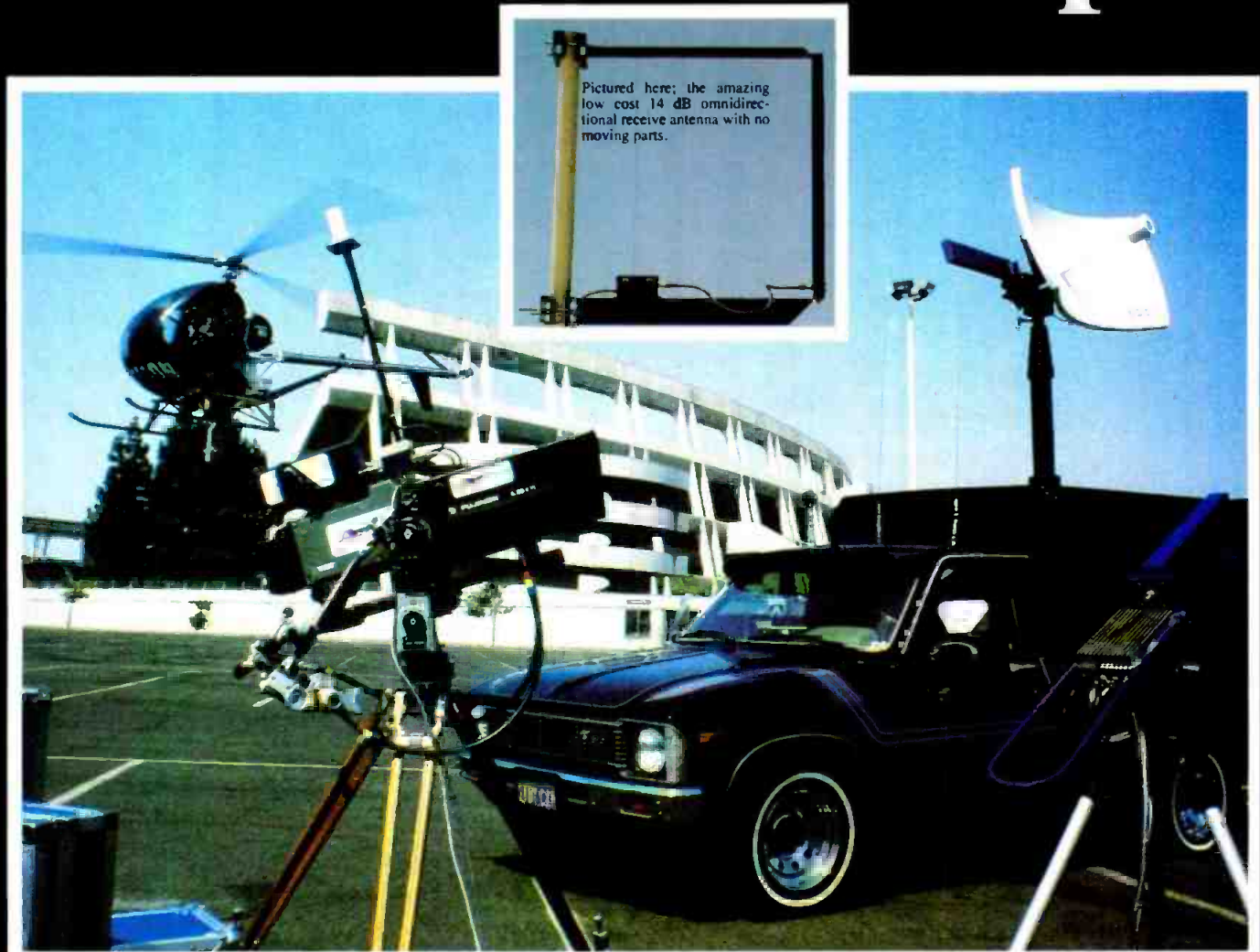
Pictured here: Hughes 300 and BMS microwave, camera mounted omni and transmitter, portable yagi antenna. Truck mounted 2x4 dish.
