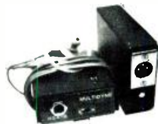
Low distortion earphone amplifier, low power, lightweight, two gain ranges, low battery flashing indicator. It can amplify telephone audio through magnetic pick-up. It costs only $110.
